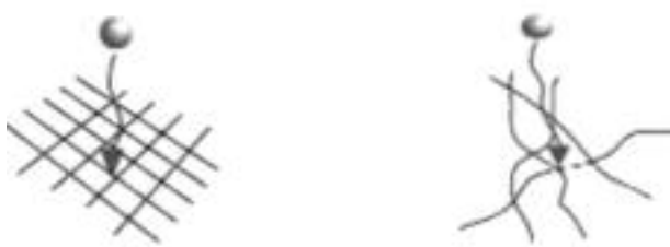
Fig. 1. Physical sieving of particulate material versus Electrostatic attraction of particulate material (Traditional theory)
